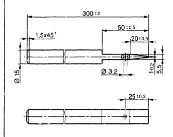
Tool for pressing out needle bearing in armature
